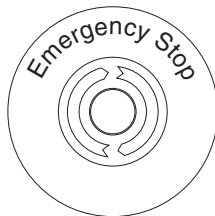
Figure 19. Emergency Stop Switch
